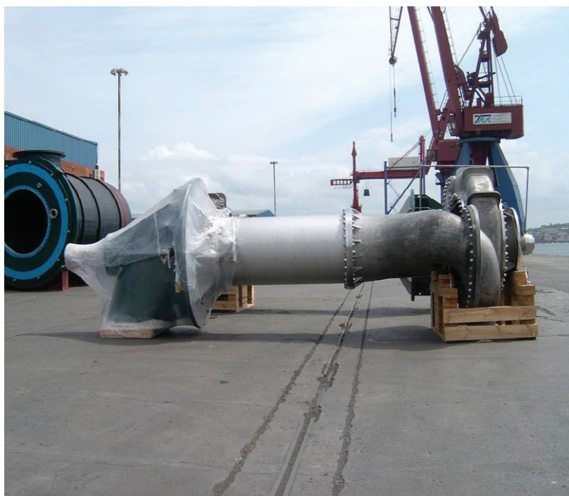
Figure 1. This brine recirculation pump is for installation in a major MSF plant in the Middle East. The pump is more than 7 m long, with a diameter greater than 4 m.
