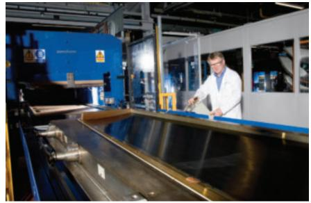
Bombardier has developed and patented its own resin transfer infusion (RTI) process for the CSeries wing.
