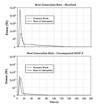
Fig. 9 – Relative contribution of pressure work and heat of adsorption for MaxSorb<sup>™</sup> and MOF-5<sup>™</sup>. System configuration and operating conditions are those of Fig. 7.
