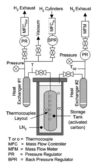
Fig. 1 – Schematic of UQTR experimental apparatus. As shown, the experiment is set up for low temperature tests. Liquid nitrogen is replaced with water or air for the high temperature tests.
