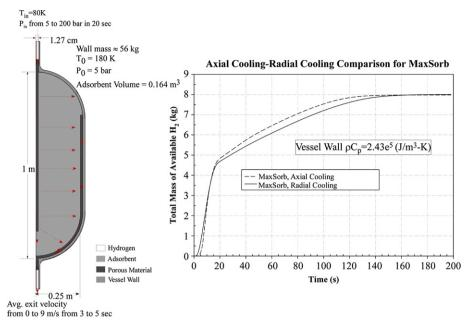
Fig. 8 - Comparison of charging rates for radial and axial flow-through cooling of MaxSorb.
