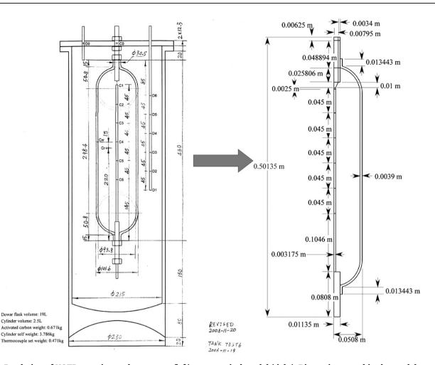
Fig. 2 – Rendering of UQTR experimental apparatus (left) as numerical model (right). Dimensions used in the model are shown in figure on the right. The total volume of the storage vessel was 2.5 L and contained 0.671 kg of MaxSorb™.
