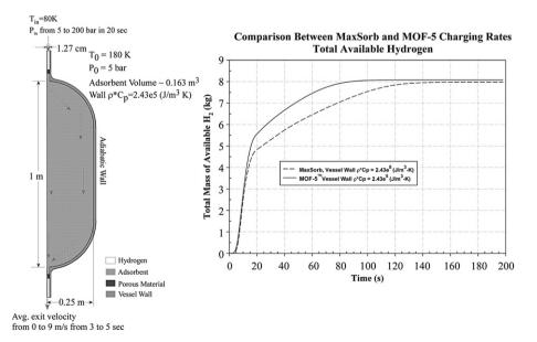
Fig. 7 - Comparison of charging rates for axial flow-through cooling of MaxSorb and MOF-5<sup>TM</sup>.
