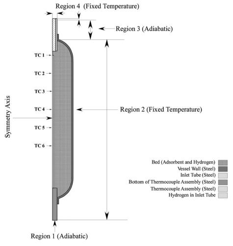
Fig. 3 - Material composition and boundary conditions used in model.
