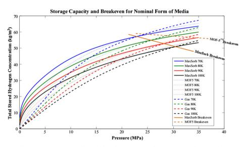
Fig. 10 – Storage capacity and breakeven curves for MOF-5™ and MaxSorb.
