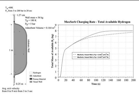
Fig. 6 – The effect of vessel wall heat capacity on charging rates for axial flow-through cooling of MaxSorb. The term 'available hydrogen' refers to the amount of hydrogen released upon return to the initial state.
