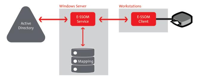
The E-SSOM Client that has been installed on the workstation is integrated directly with the card reader's driver software. It can send queries to the card reader such as 'Is the card placed in the reader?', 'Is the card near the reader?', 'What is the card's RFID?''. E-SSOM can also respond to any event generated by the card reader, e.g. when the card is held near the reader.
