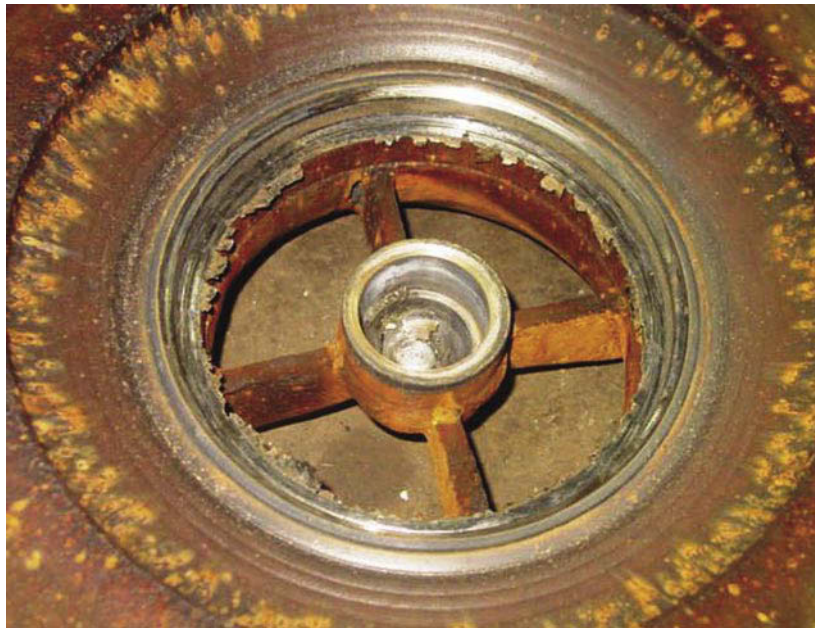
Figure 4. Damage to first-stage casing, wear ring and bottom bush.
