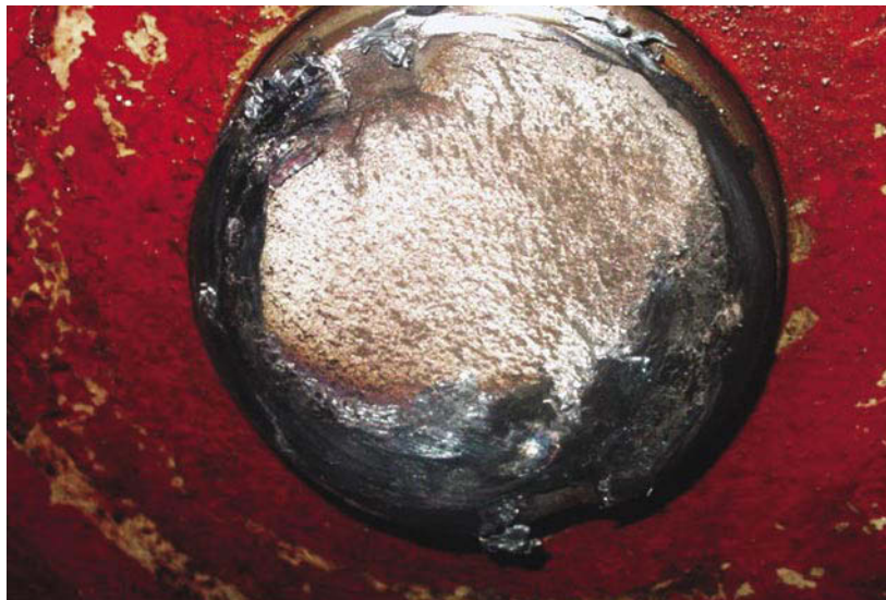
Figure 7. The fatigue fracture surface of the motor shaft.
