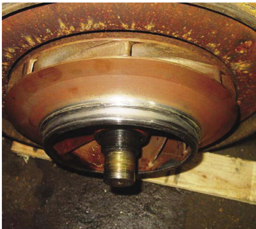
Figure 5. Damage to first-stage impeller front shroud and wear ring.
