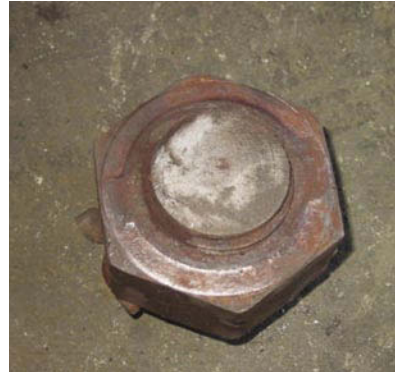
Figure 3. Appearance of pump shaft fatigue fracture surface.
