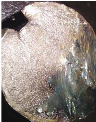
Figure 6. Fracture location on the motor shaft immediately behind the coupling core.
