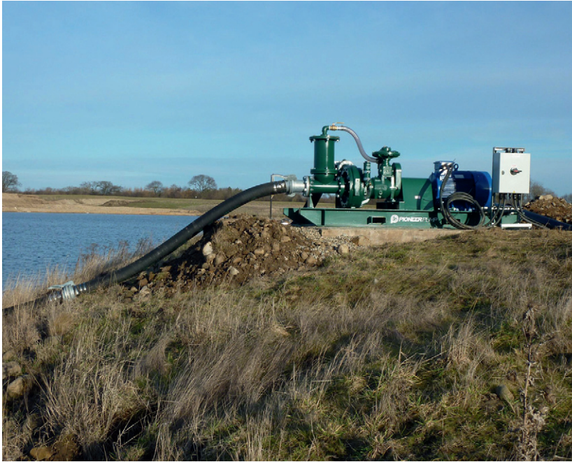
Figure 3. A PP64S17 pump electric (WEG) motor-driven is pumping 300 m 3 /hr to an 80 m head.
