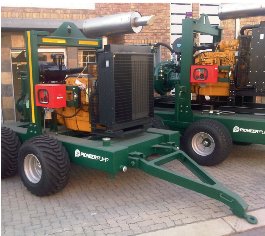
Figure 7. John Deere engine powered Pioneer pumps mounted on trailers.
