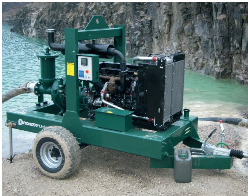
Figure 1. A PP64S17 pump Perkins 1106-driven quarry trailer in Doveholes, Buxton, UK. This, delivered to Cemex, pumps 350 m 3 /hr at a 62 m head maximum. It operates as a feed pump to a washplant.
