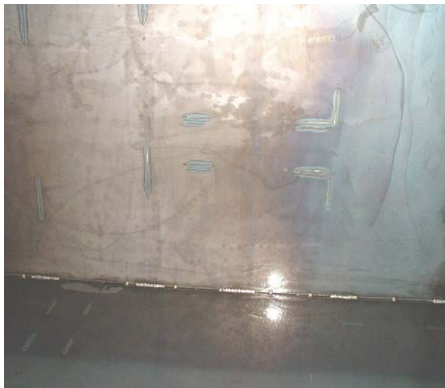
Figure 2. Image of the dump bed after the pressure wash. Notice how the contaminants are gone and the metal is taking on a bluish color. This is from the warm phosphate.
