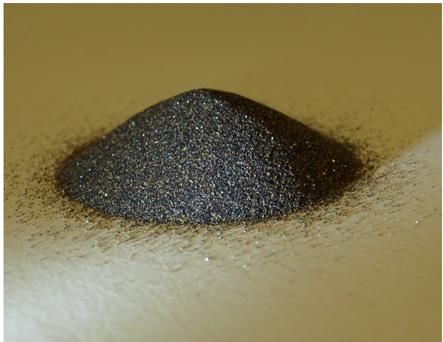
Figure 3: The oxide powder which is turned into metal powder in a single step.
