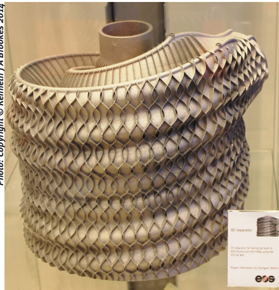
Figure 14: An oil separator for a racing car built in an EOS M400 from EOS Aluminium AlSi10Mg powder.
