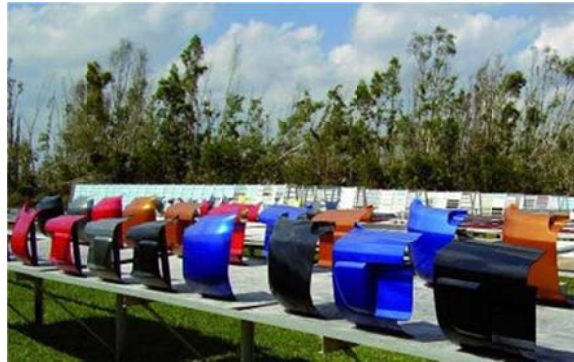
Figure 8: Weathering rack at Atlas' facility in Florida with various car body parts
