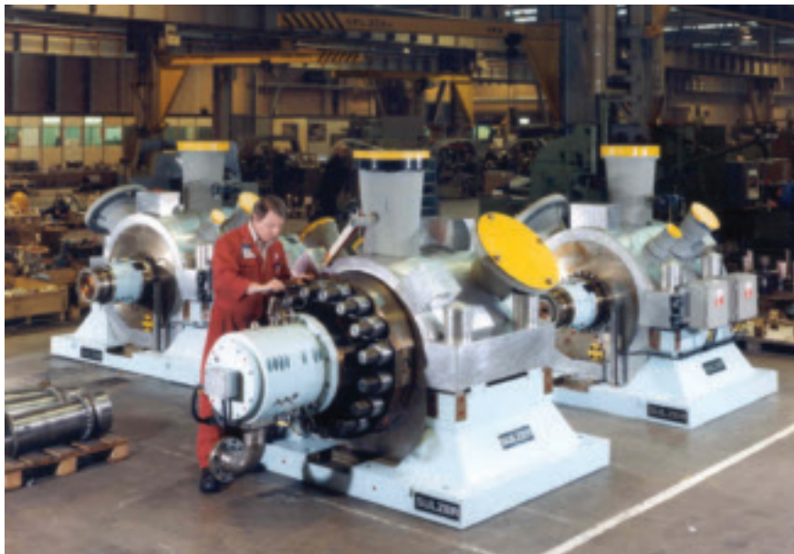
Figure 1. Newly built Sulzer boiler feed pumps.
