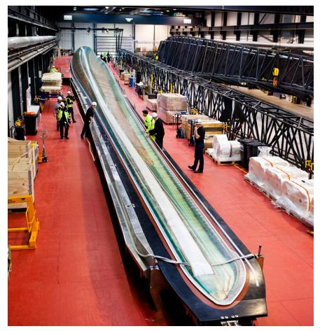
Siemens manufactures the blades in one piece using its IntegralBlade process.
