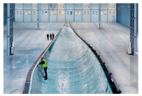
The mould for the B75 blade consists of two parts.
