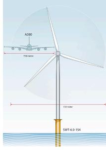
The 75 m blades will be used on Siemens' 6 MW (SWT-6.0-154) offshore wind turbine. This turbine can also be equipped with a 120 m rotor, standard equipment for the Siemens 3.6 MW offshore turbine, to allow the 6 MW turbine to be installed in locations where air traffic regulations dictate a maximum tip height of 150 m.
