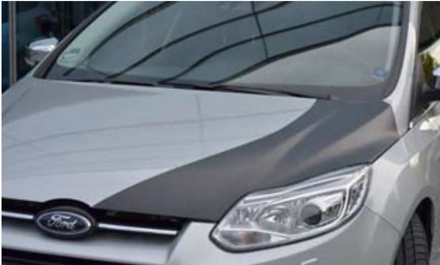
Ford has developed a carbon fibre bonnet for the Ford Focus. It says production time for an individual carbon composite bonnet is fast enough to be employed on a production line. (Picture © Ford Motor Company.)
