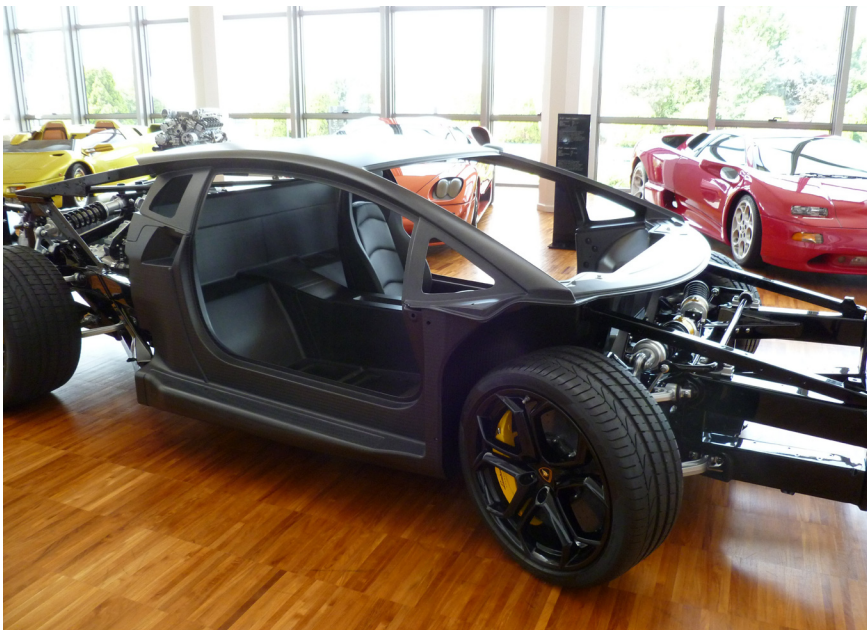
The Aventador (top picture), launched in 2011, is built around a carbon fibre reinforced plastic monocoque (lower picture), manufactured in-house at Sant'Agata by Lamborghini.
