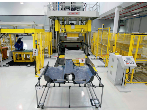
Part of the RTM line.
