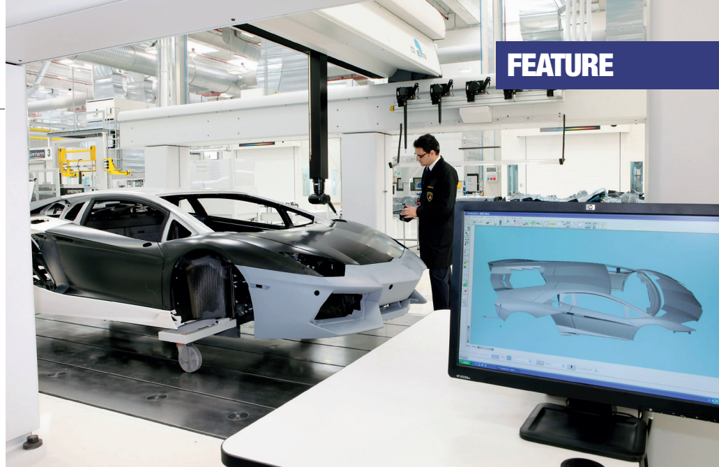
Final checks ensure exact tolerances are met.
