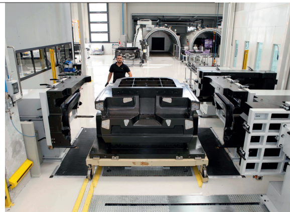
The autoclave room, where prepreg components are cured.
