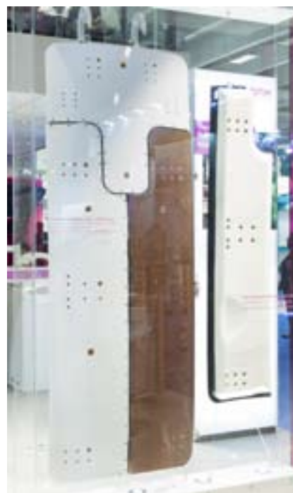
Nose gear door made using ROHACELL HERO foam core material.
