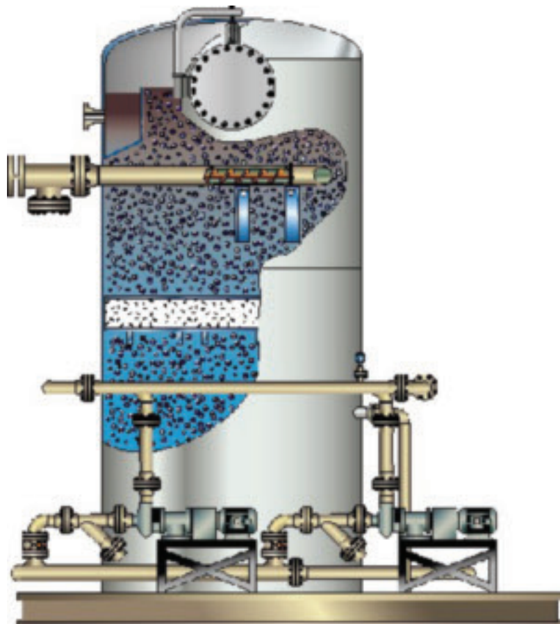
Figure 4: Dissolved gas flotation unit. (Courtesy of Siemens Water)
