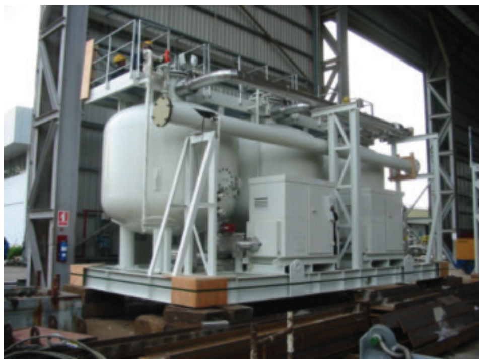
Figure 9: Dual media seawater filters. (Courtesy of Cameron Process Systems)
