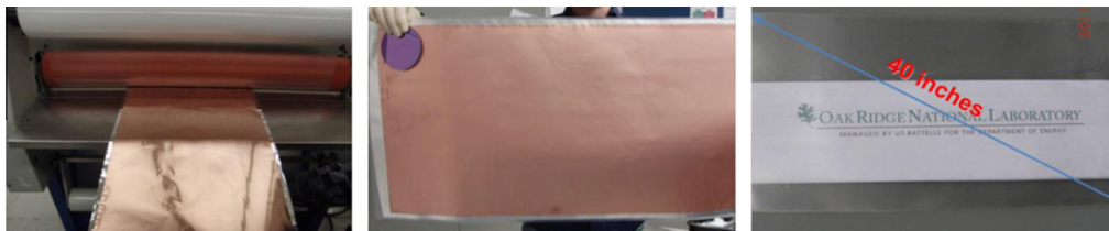
Fig. 7 – Transfer of graphene films on flexible, transparent PET polymer: lamination of copper foil with graphene by PET polymer; laminated sample, 4" wafer is shown for comparison; Example of 40" graphene film on PET polymer prepared by atmospheric pressure CVD synthesis with sheet resistance 1–3 k \Omega /sq.
