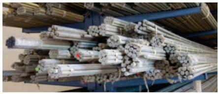
C-Bar composite reinforcing bar from Marshall Composites is said to exhibit 1.5 times the tensile strength of steel at one-quarter the weight.
