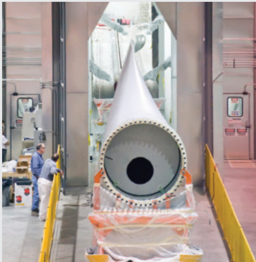
A wind turbine blade positioned in the automated paint facility in an MFG blade manufacturing facility. (Picture courtesy of MFG.)
