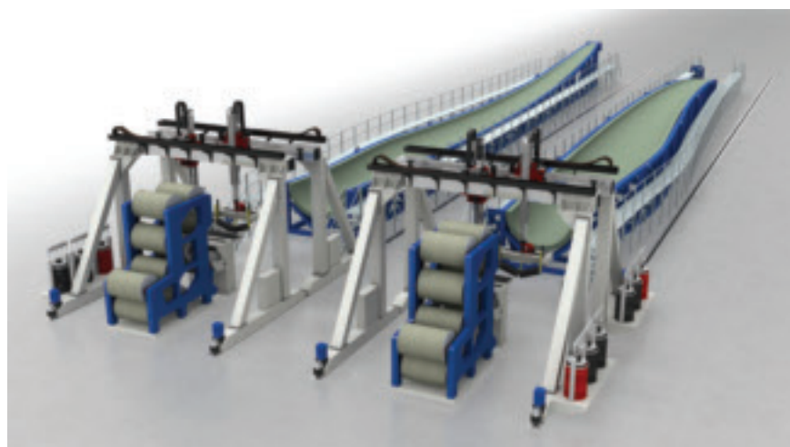
The MAG Rapid Material Placement System automatically sprays in mould coatings and cuts and lays in glass and carbon fibre materials. (Picture courtesy of MAG IAS.)
