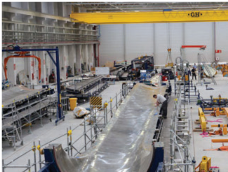
A mould is prepared for infusion of a blade shell-half at Gamesa's wind blade manufacturing plant in Navarra, Spain. (Picture courtesy of Gamesa.)
